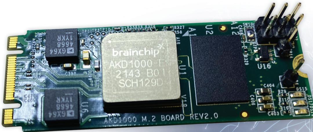
**Fig.5** The BrainChip AKD1000 evaluation board contains the Unified Convolutional Neuromorphic chip. BrainChip also provides a free tool called MetaTF™ that integrates seamlessly with popular frameworks to allow developers to build and deploy AI smoothly. More information is available on BrainChip’s Website. <https://brainchip.com/akida-enablement-platforms/>
