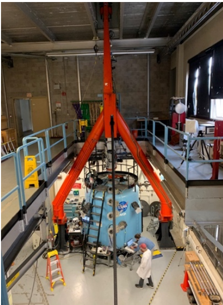
Fig. 6. Presents a photo of the AVGR facility, the blue structure is the vacuum chamber, the orange structure raises and lowers the gun. (Photo credit NRL/A. Nicholas).
