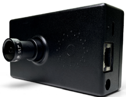
Fig. 14. The Prophesee 4.1 HD neuromorphic camera.
