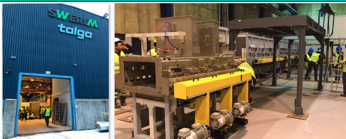
Figure 10 - TLG Electric Vehicle Anode (EVA) plant and installation of EVA anode coating kiln
