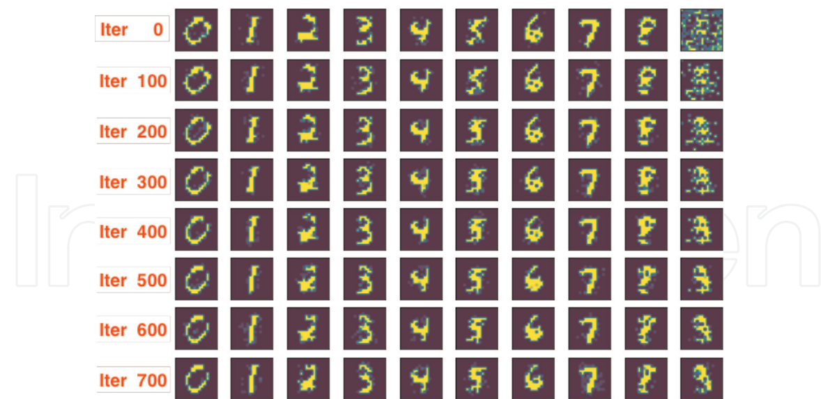
Figure 11. Online incremental learning: A single TNN mini-column trained only on the digits 0–8 learns a new previously unseen digit ‘9’ within 500 samples (that consist about 50 samples of digit ‘9’) in an unsupervised manner [11]. This demonstrates the online learning capability of TNNs, which can quickly learn new classes from relatively few examples without forgetting previously learned information.
