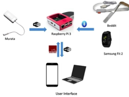
Figure 1. Architecture of the sleep monitoring system
